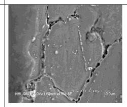
Cavitation in surface section
